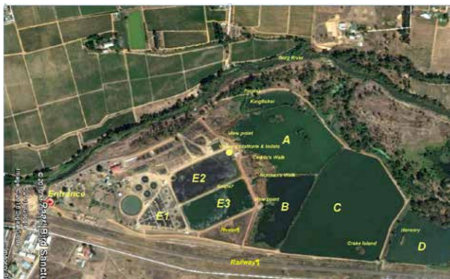
Paarl Bird Sanctuary is bordered by the Berg River and vineyards to the west, with industrial and residential areas to the east. Pans A–D form an artificial wetland that attracts prolific birdlife, and from which treated waste water feeds back to the river for reuse downstream
