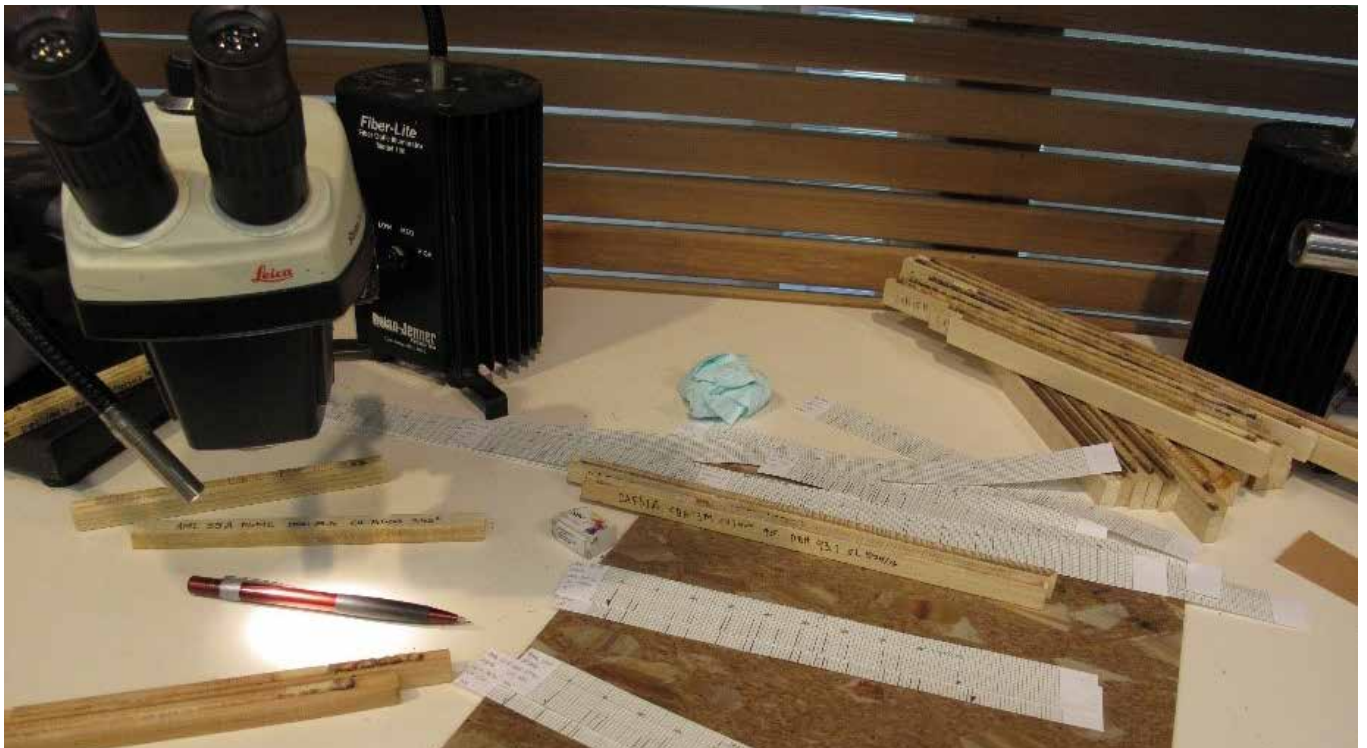
Analysing the cores using skeleton plotting in an attempt to build a master chronology for a sampling site
